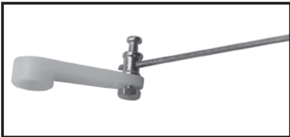
CONTROL HORN OF THE AILERON
